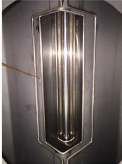
Figure E-6. View of the surrogate SNF basket and thermocouple through a viewport. (Knight et al. 2019).
