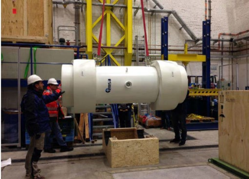
Figure H-13. Photo of the 1/3 Scale ENSA ENUN-32 cask with impact limiters. (Kalinina et al. 2019)
