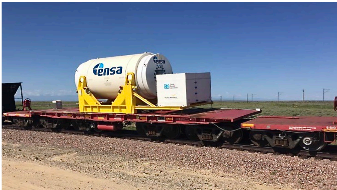
Figure 3-6. Multimodal Transportation Test cask on a railcar.
