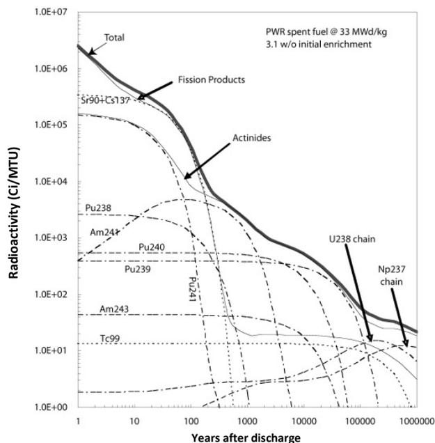
**Figure 7. Radioactivity (Curies per Metric Ton of Uranium) vs. Time for Pressurized Water Reactor Spent Nuclear Fuel.** Reproduced from Xu et al. (2005) with Permission from the American Nuclear Society, La Grange Park, Illinois.
