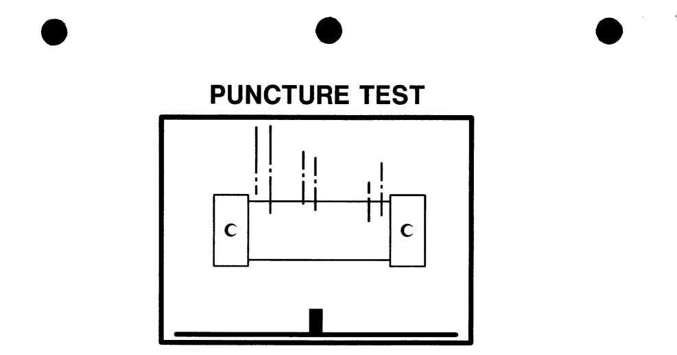
FORTY INCH FREE DROP ONTO A 6 INCH DIAMETER MILD STEEL BAR AT LEAST 8 INCHES LONG IN A POSITION FOR WHICH MAXIMUM DAMAGE IS EXPECTED.
