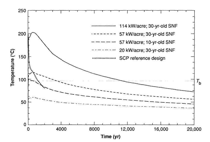
Temperature history along the repository centerline for various thermal loading conditions at the repository horizon.
