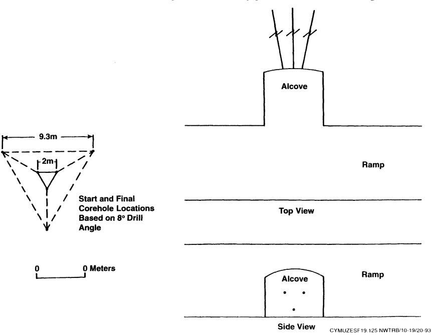
Test description: Air-permeability anisotropy testing
