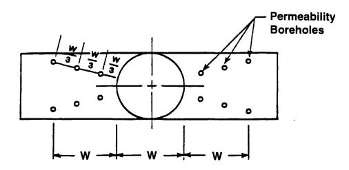
W = Excavation Diameter (Or Width)
