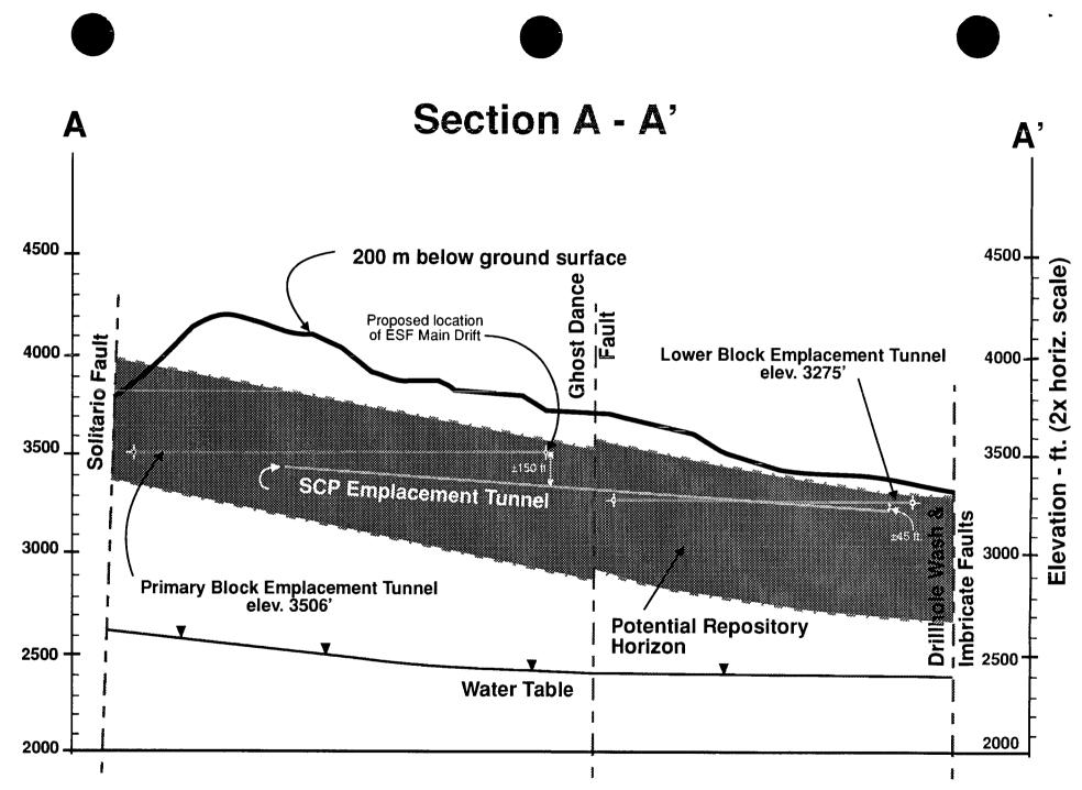
Note: Plane of section cuts through lowest emplacement drift in working concept layout.
