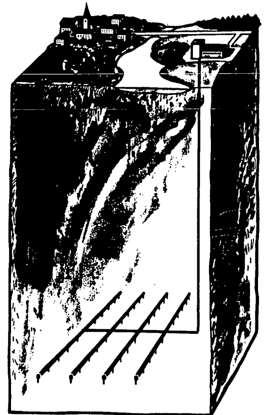
Deep geological repository for spent nuclear fuel. First stage of deposition 2008 at the earliest.
