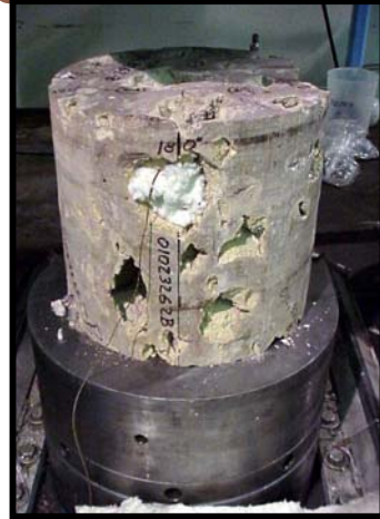
Uniaxial Compression Test on a Sample at 200 deg C (8/02)
