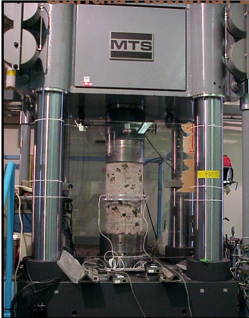
Uniaxial Compression Tests of the 11.5" diameter upper lithophysae samples (7-8/02)
