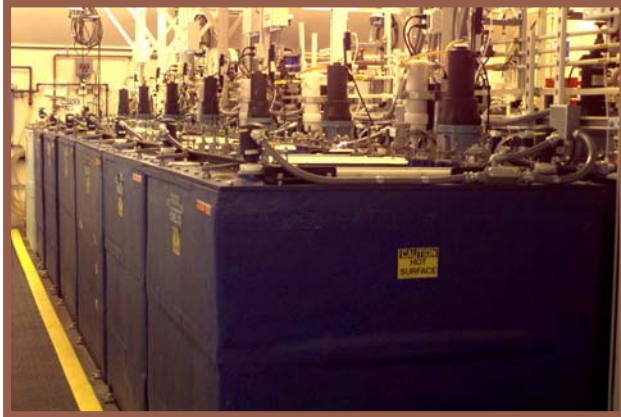
Thousands of waste package samples are exposed to repository-relevant conditions in the Long Term Corrosion Test Facility
