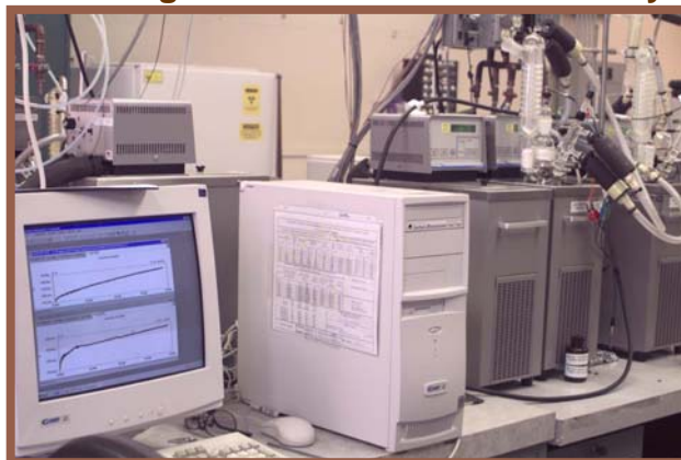
Arrays of potentiostats are used to measure threshold potentials for localized corrosion and the time-evolution of the corrosion potential
