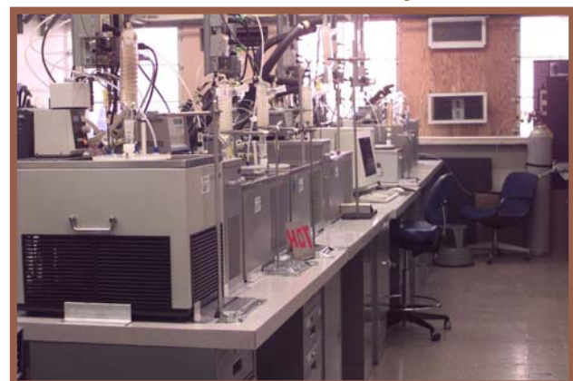
Arrays of potentiostats are used to measure threshold potentials for localized corrosion and the time-evolution of the corrosion potential
