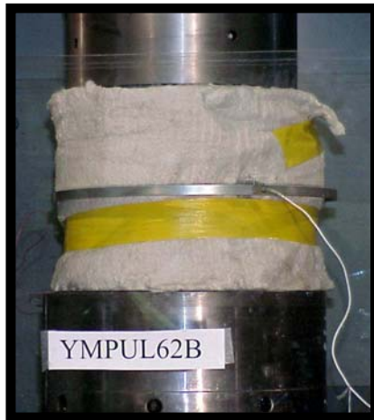
Uniaxial Compression Test on a Sample at 200 deg C (8/02)
