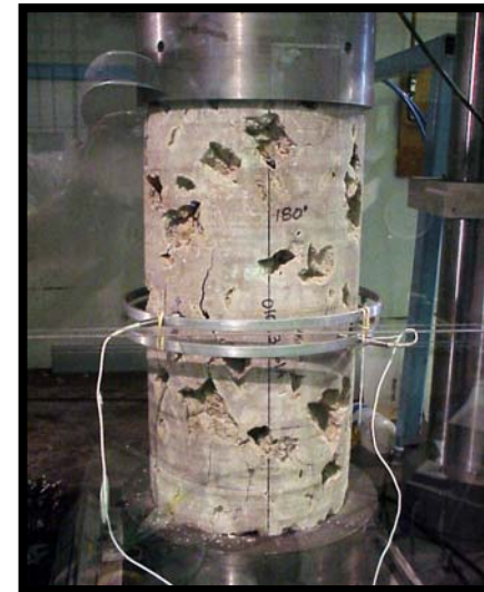
Uniaxial Compression Tests of the 11.5" diameter upper lithophysae samples (7-8/02)
