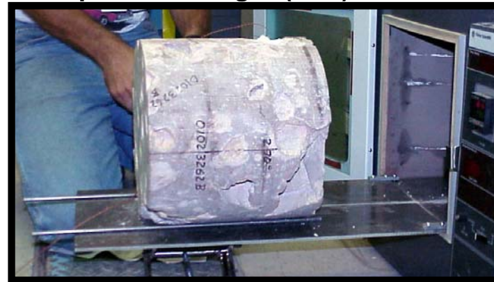
Thermal Expansion Test Sample (8/02)
