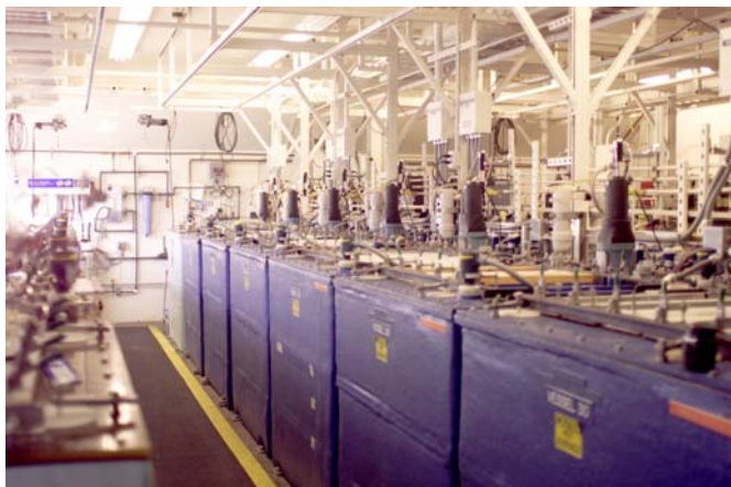
Immersion Testing ASTM G 31 Long Term Corrosion Test Facility (LTCTF)
