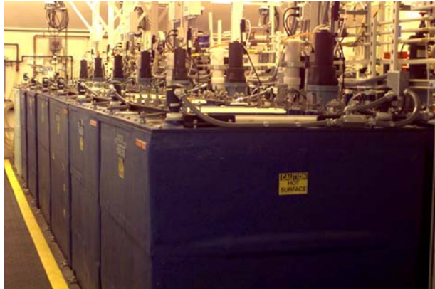
Thousands of corrosion samples are exposed to high-temperature saturated brines in the Long Term Corrosion Test Facility
