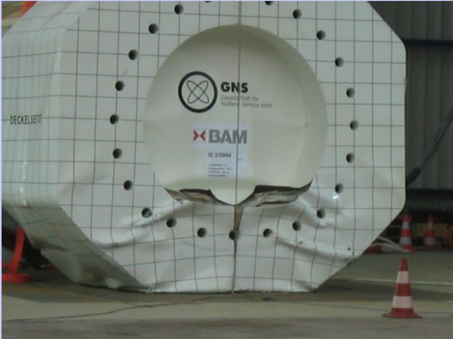
End view after 9-meter side drop test
