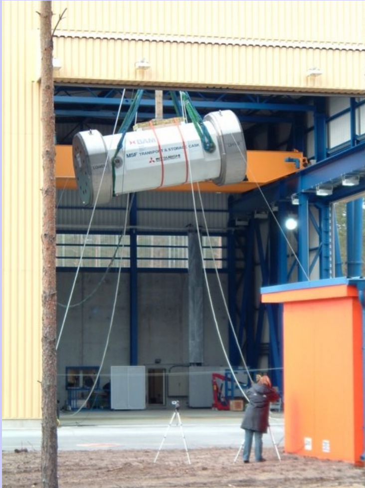
Test preparation for MHI-MSF69 BG Spent Fuel Cask (shallow angle drop)
