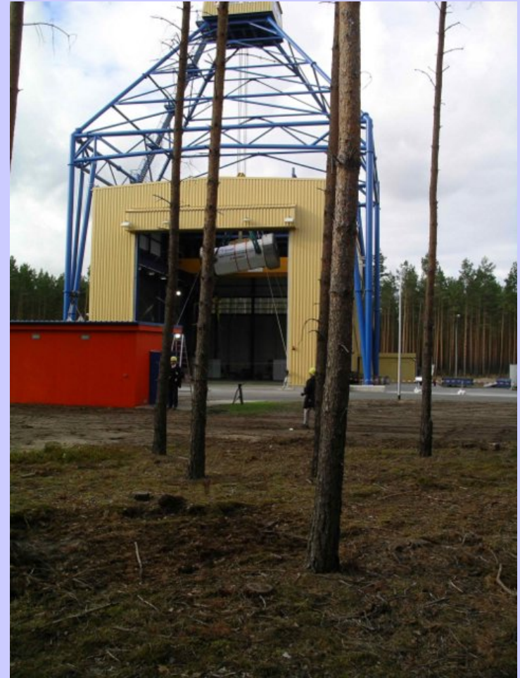
Test preparation for MHI-MSF69 BG Spent Fuel Cask (shallow angle drop)
