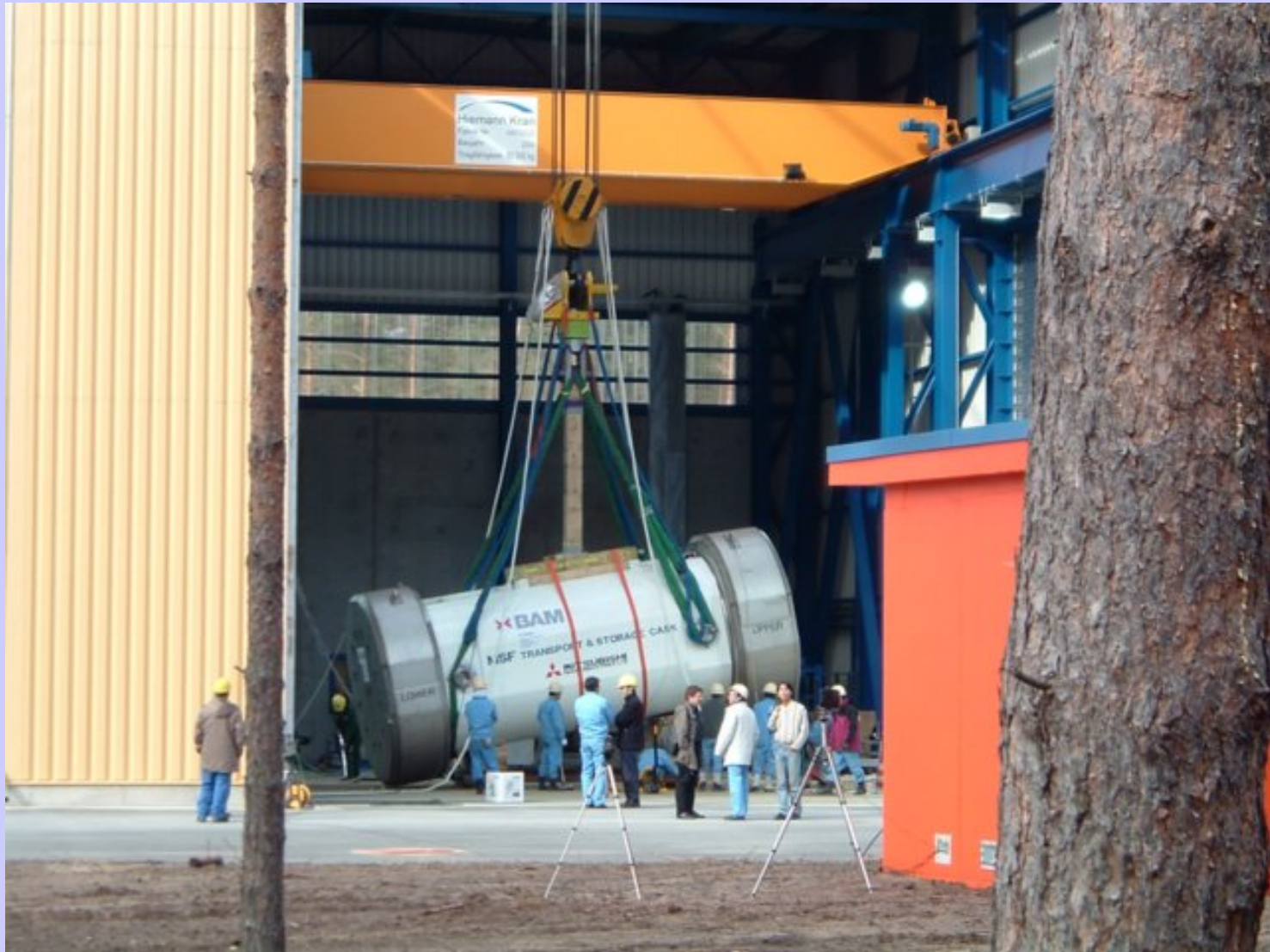
MHI-MSF69 BG Spent Fuel Cask being prepared for shallow angle drop test
