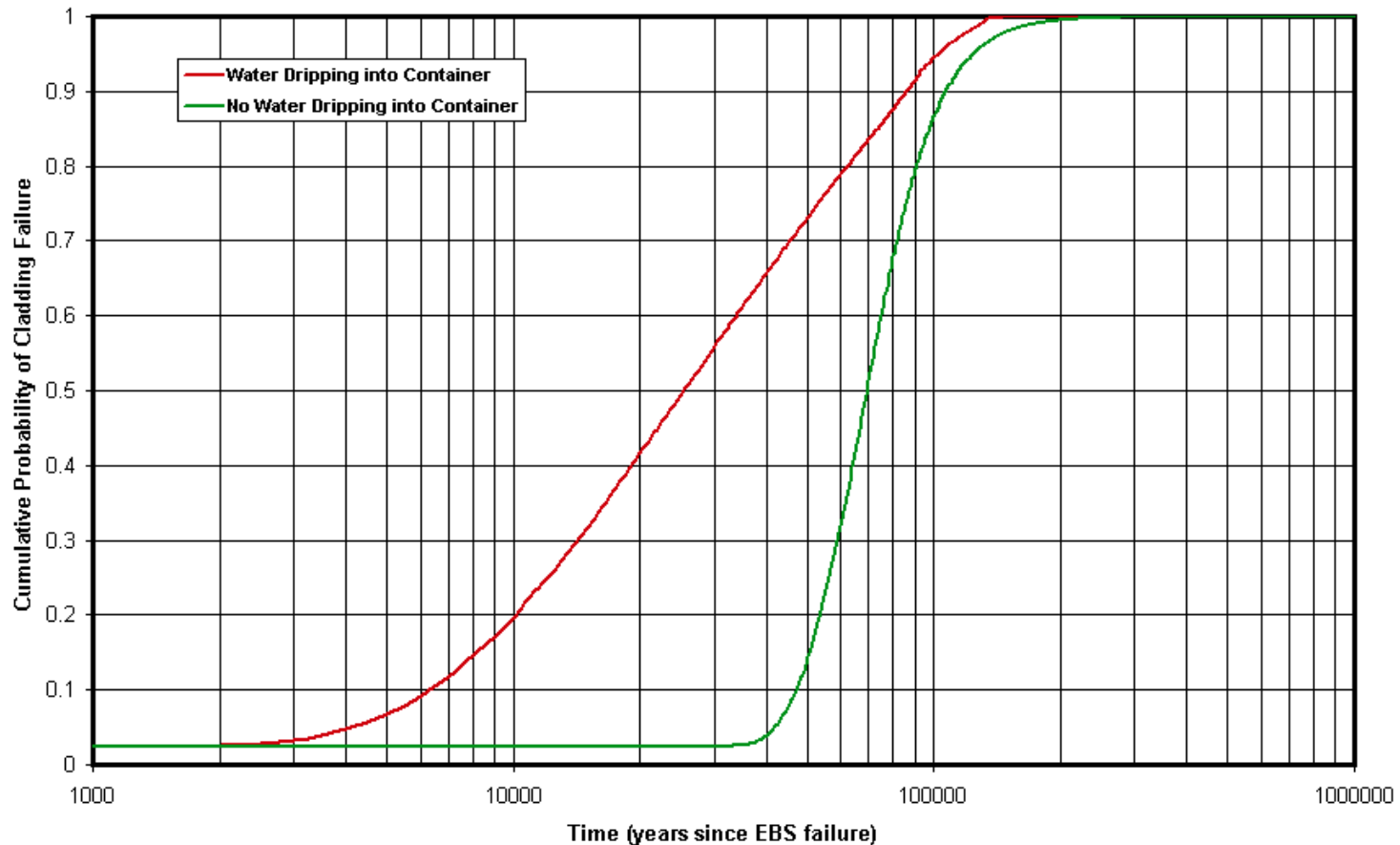
Wet / Dry Cladding Failure Distributions
