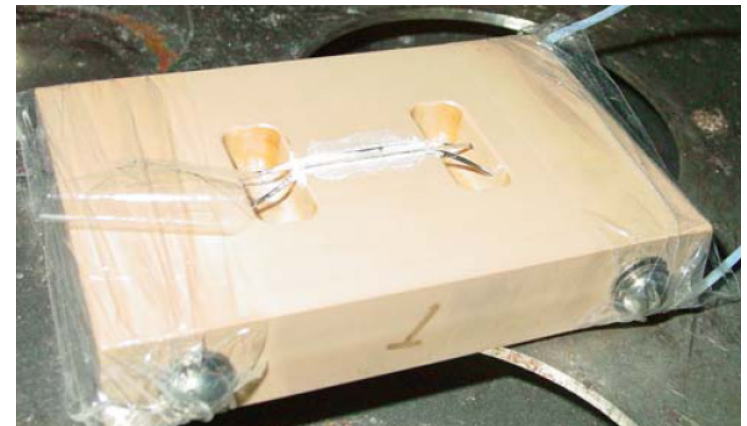
Parallel Pt wires used to detect deliquescence of salt assemblage
