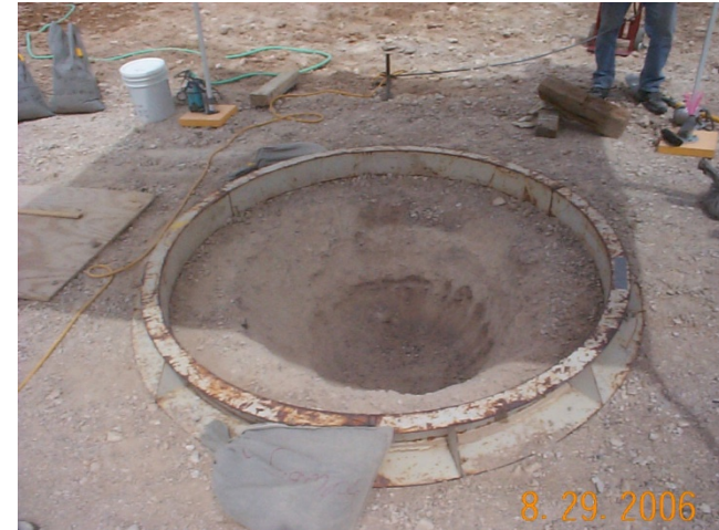
Ring Density Test Being Performed in a Test Pit
