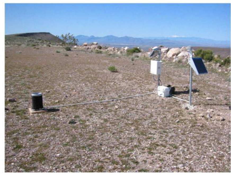
Left: Location of six precipitation sites around Yucca Mountain. Above: Typical precipitation site showing tipping bucket gauge, storage module, and data logger.
