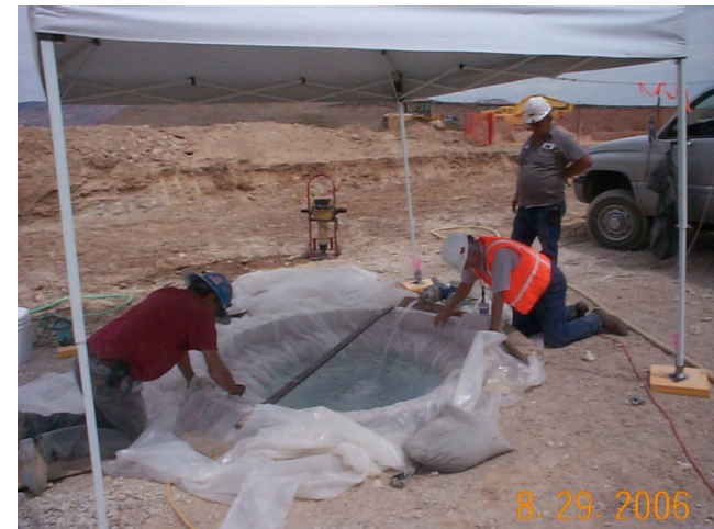
Ring Density Test Being Performed in a Test Pit
