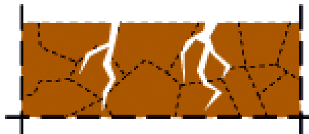
Stress corrosion cracking
