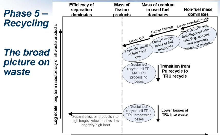
Log scale: disposed mass that has both high long-term radiotoxicity and high heat
