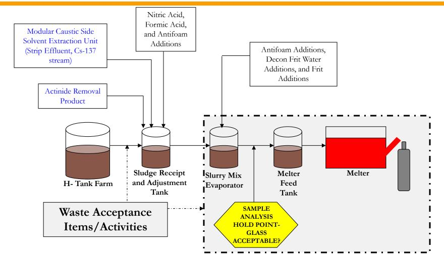
Process works to produce highly durable borosilicate wasteform.
