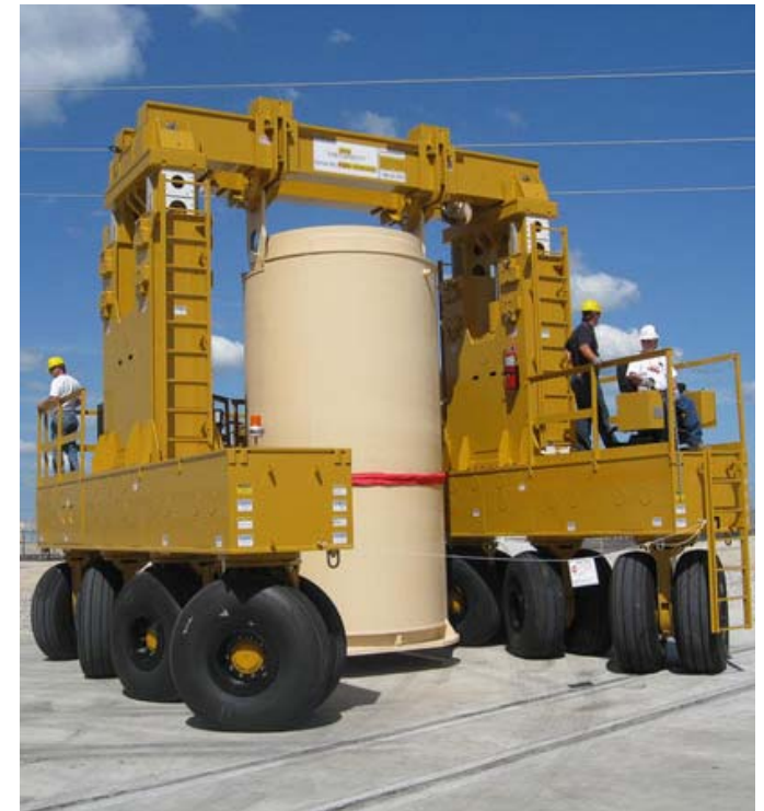
Wheeled cask transporter used to place a cask on a storage pad
