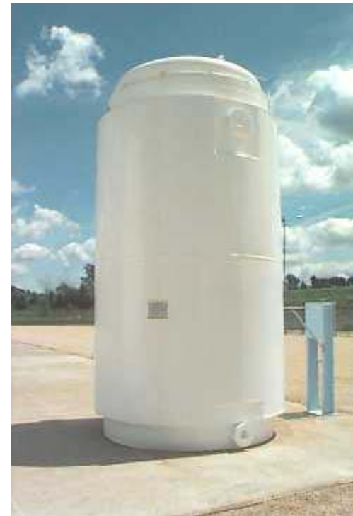
Metal Storage and Transportation Cask similar to what will be loaded
