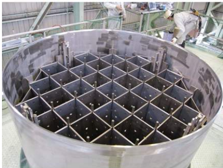
Empty canister showing baskets for UNF assemblies
