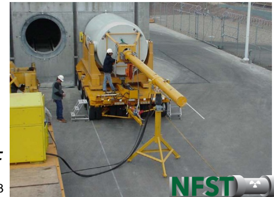
Transnuclear Horizontal Storage Module
