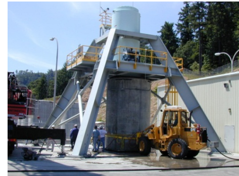
Loading canister into storage overpack at Trojan using transfer cask
