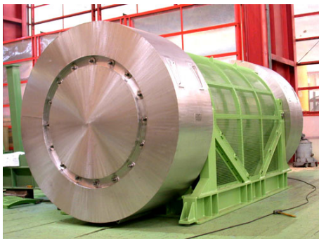
Empty canister showing baskets for UNF assemblies
