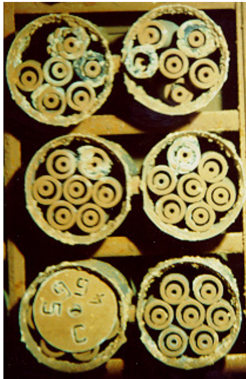
Top Left: Damaged N Reactor Fuel Element.
