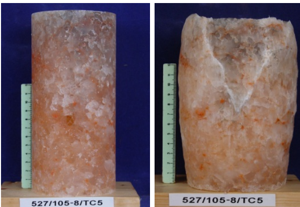
Room Temperature Triaxial Test Sample of WIPP Salt at 3.0 MPa Confining Stress
