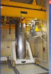
Waste canisters pulled from shipping cask behind shield doors and placed into shielded facility cask for handling
