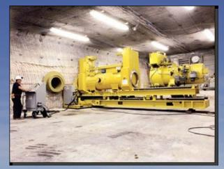
RH waste in the canister is emplaced in pre-drilled boreholes in disposal room walls, and a concrete shield plug is inserted afterwards
