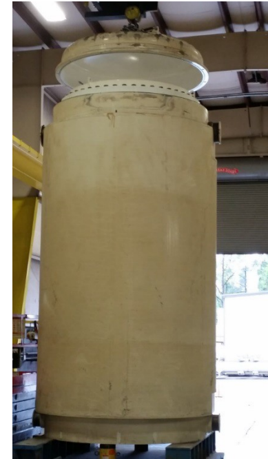
Removing lid to inspect cask after years of storage
