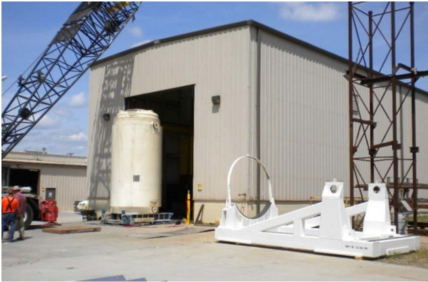
TN 32B cask at fabricator
