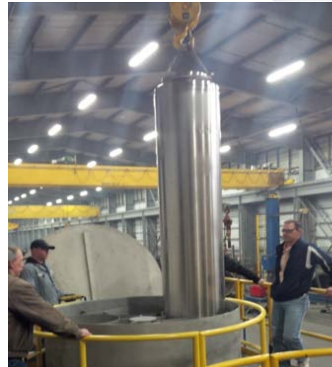
West Valley High Level Waste Canister Test Fit In Overpack
