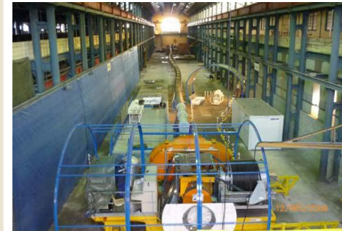
Test to retrieve a waste package from a distorted disposal cell
