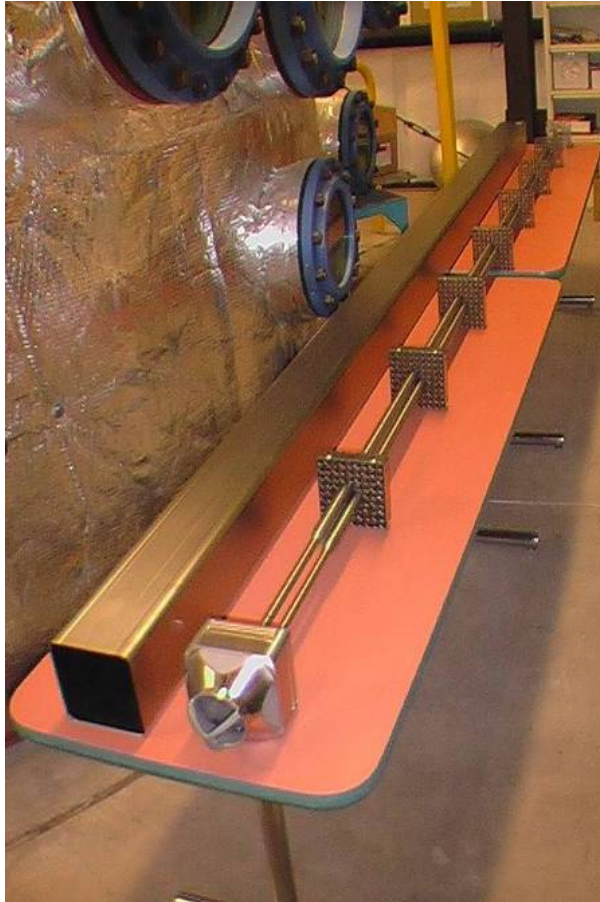
BWR channel, water tubes and spacers
