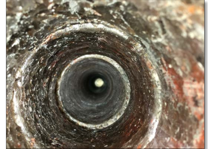
Discrete fractures in BATS near-drift EDZ
