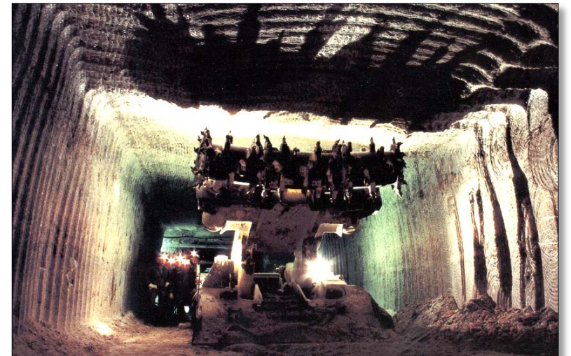
Continuous miner at WIPP
