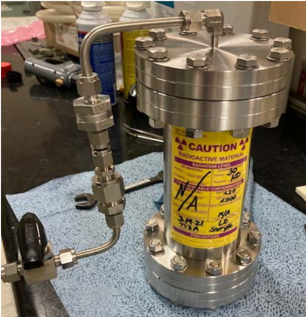
Loaded and sealed mini-canister with reactor-exposed sample
