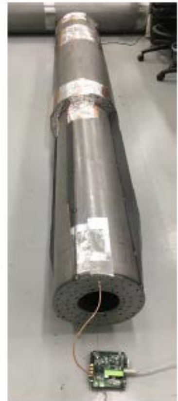
2.4 GHz transmitter connected to bottom bucket antenna
