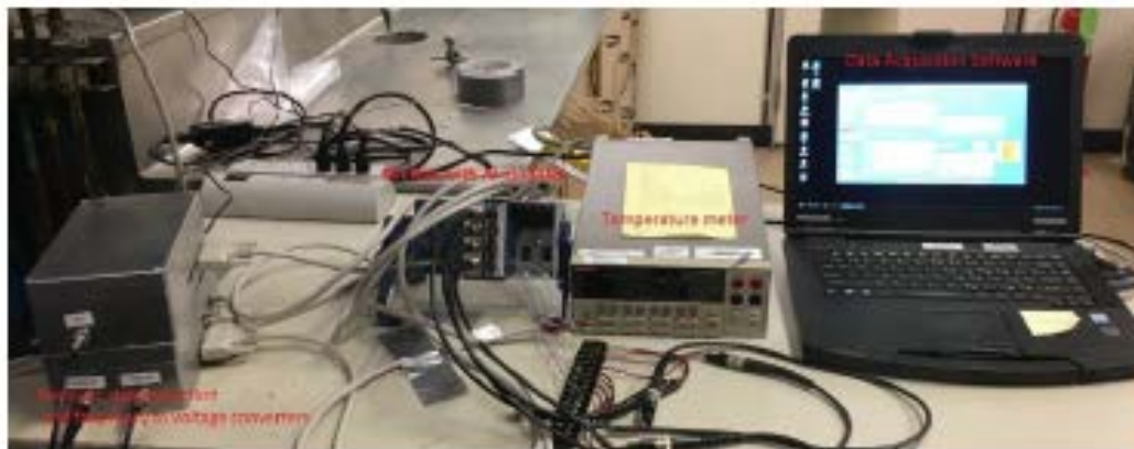
In-canister hardware irradiation data acquisition system
