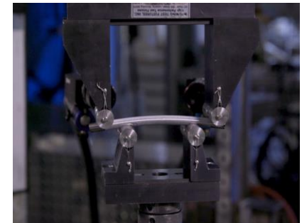
4-point bend test—apparatus located at PNNL
