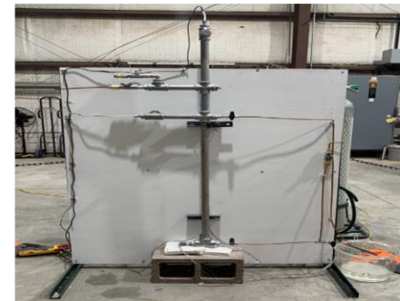
SNL Dry Storage Cask Thermal Hydraulic Testing Pressure Vessel and Mount.
