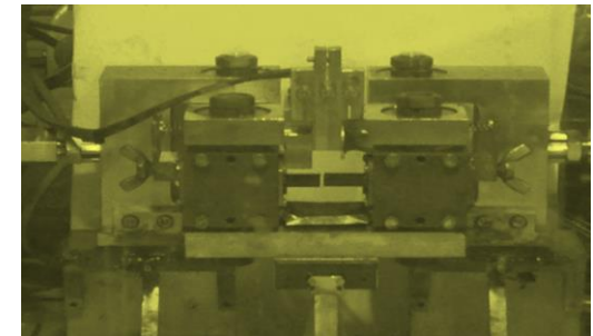
Cyclic Integrated Reversible-bending Fatigue Tester (CIRFT) located at ORNL
