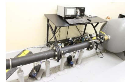
SNL test apparatus for determining efficiency of particles moving through a SCC crack and dispersion modeling.
