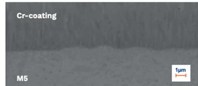
Metallographic cross-section of Cr-coated M5 Cladding tube before irradiation
