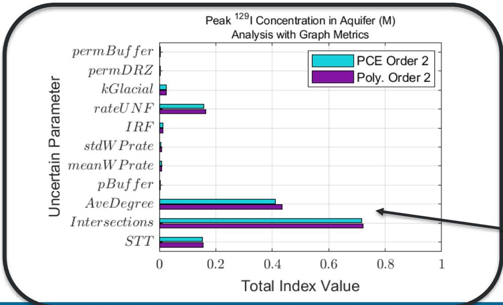
Adding graph metrics to the SA significantly changes the results, showing the influence of DFNs. The fracture network and where fractures land has a larger effect on peak 129-I than source term and EBS uncertainties.
