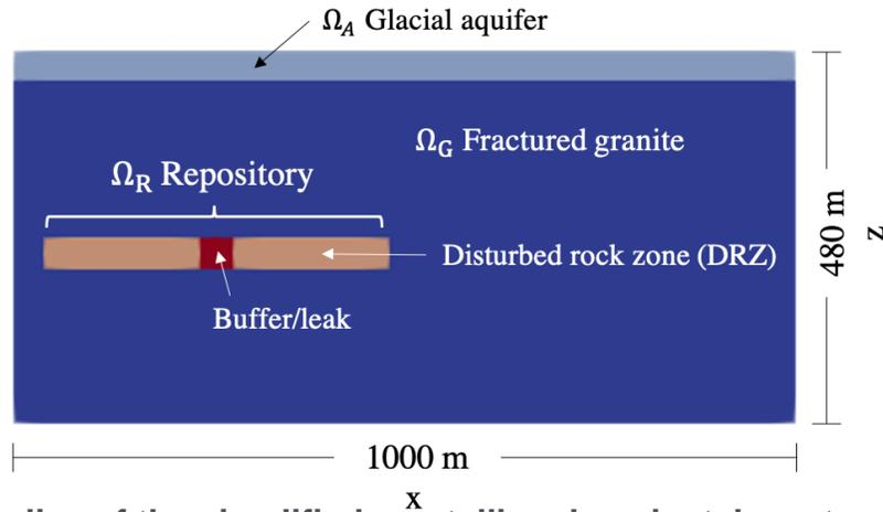
A vertical slice of the simplified crystalline domain, taken at  $y = 500$  m
