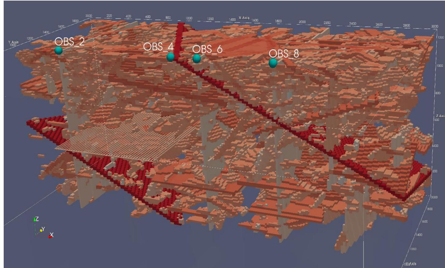
Cut-away of DFN 1 realization mapped to porous medium grid, showing the full repository and the far half of the model domain.
