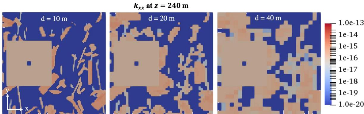
Horizontal slices of the permeability tensor in the x-direction for meshes with cell sizes  $d = 10, 20,$  and  $40$  m, from left to right.
