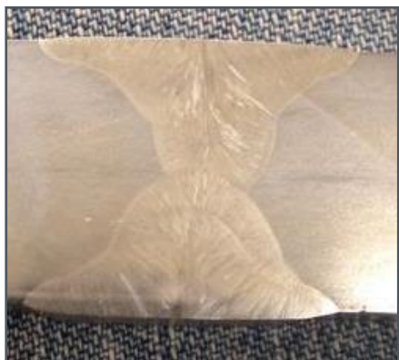
Weld zone, Ranor 304 SS plate
