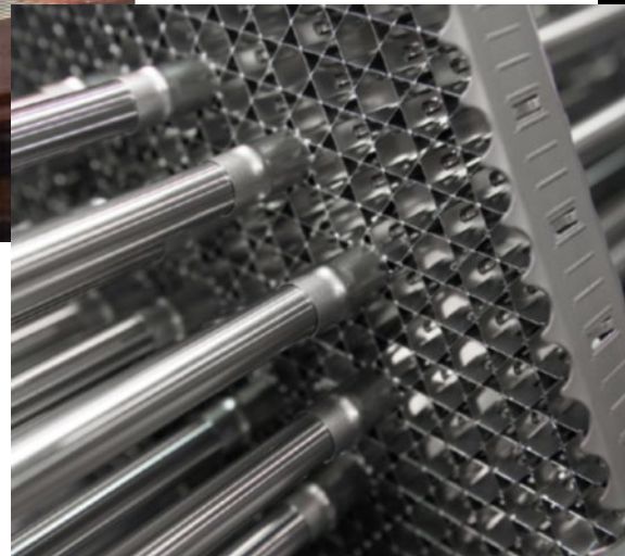
Example grid spacer showing thin-walled cells
