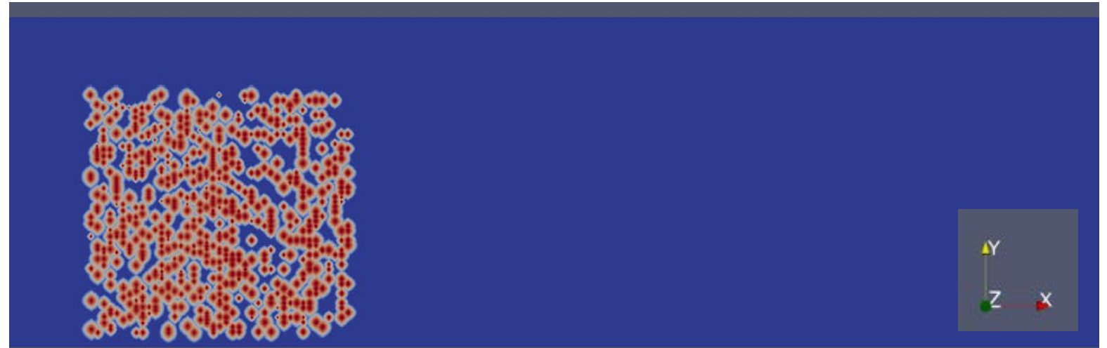
I-129 concentration at 10,000 y plotted in a horizontal slice at the Z-midpoint of the repository.
