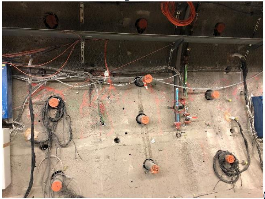
Borehole array on tunnel wall
