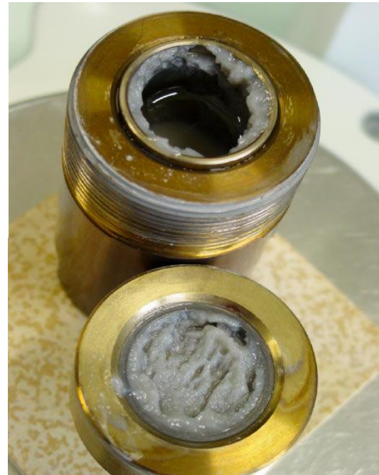
Details of titanium autoclaves and mounting arrangement of autoclaves in the oven (Leupin et al. 2014)
