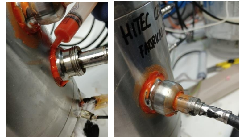
Sealing of sensors' inlets with high- T -resistant silicone
