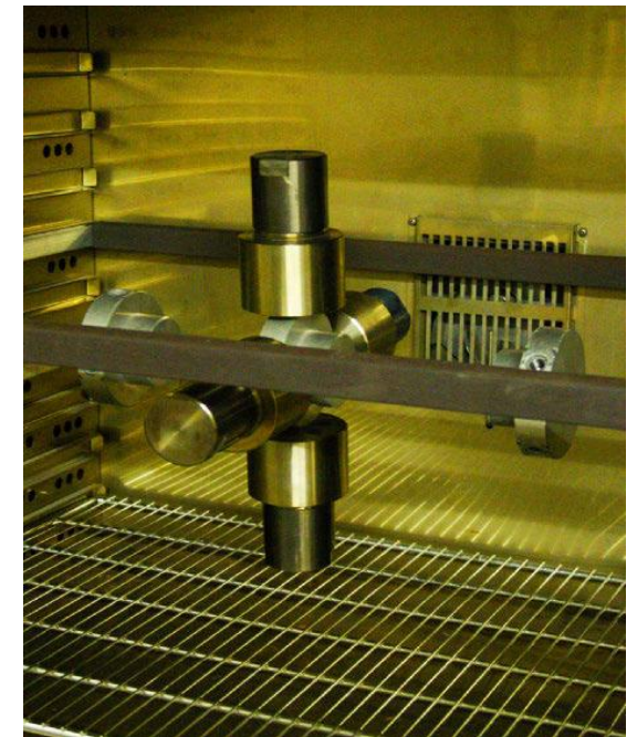
Details of titanium autoclaves and mounting arrangement of autoclaves in the oven (Leupin et al. 2014)
