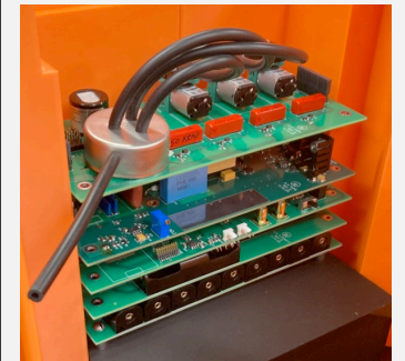
Canister lid system in 3D-printed mock-up enclosure [19].
