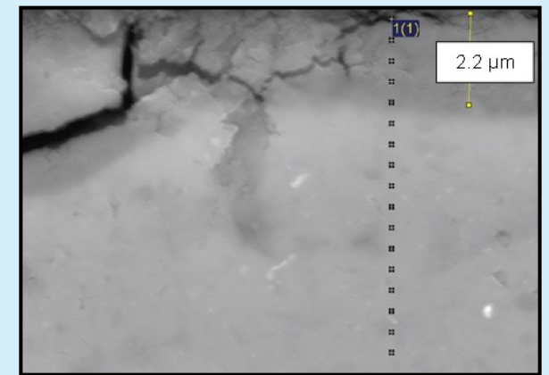
Scanning electron microscopy of an ATR (oxy)hydroxide layer cross section [13].
