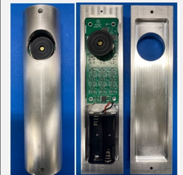
In-canister sensor mechanical assembly [19].
