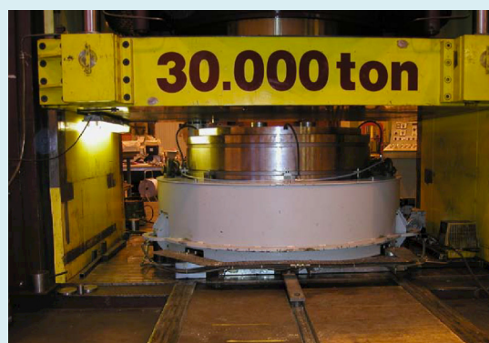
Figure 1-1. Photo of a mold SKB used for making ring-shaped bentonite blocks (SKB 2010).
