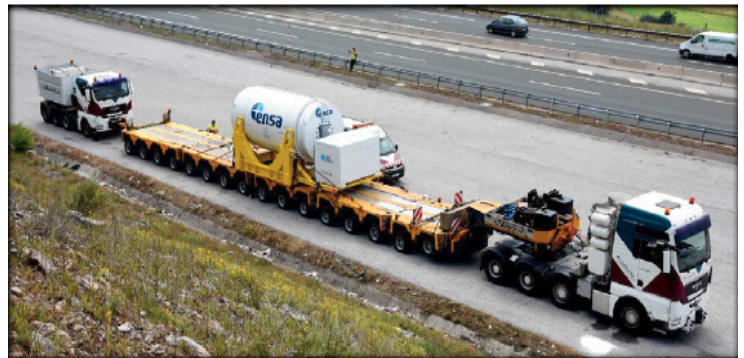
Figure A - 10. Multimodal Transportation Test; ENRESA [Empresa Nacional de Residuos Radiactivos Sociedad Anónima] ENUN-32P cask on a heavy haul truck (McConnell et al. 2018) (see footnote 81).
