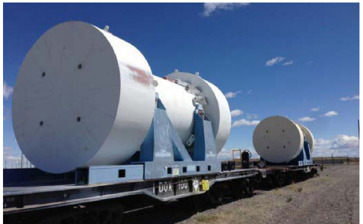
Figure A - 8. Rail transport casks (with impact limiters installed) used to transport spent nuclear fuel from the West Valley Demonstration Project Site (West Valley, New York) to the Idaho National Laboratory (Bickford 2022).
