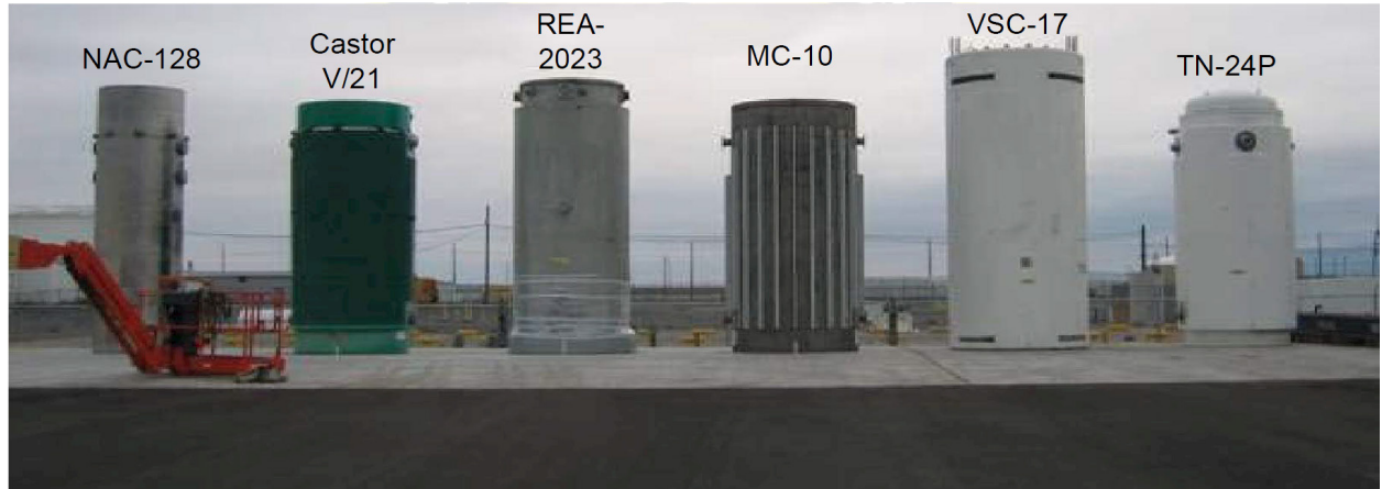
Figure A - 5. Dry-storage casks at the Idaho Nuclear Technology and Engineering Center, Idaho National Laboratory (Hanson et al. 2012).
