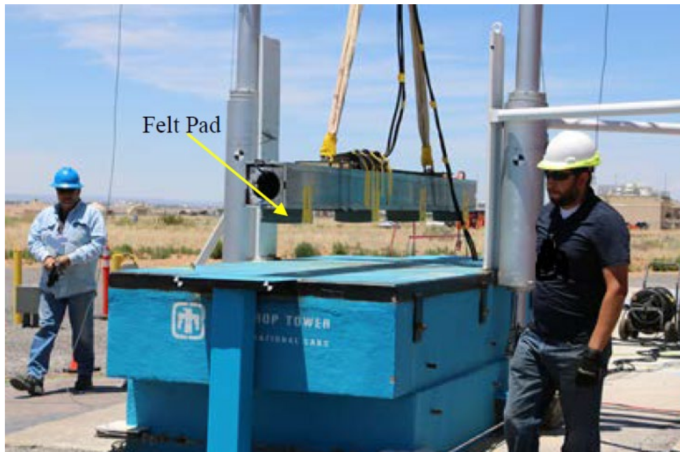
Figure H-15. Full-Scale Dummy Assembly Drop Test Setup.
