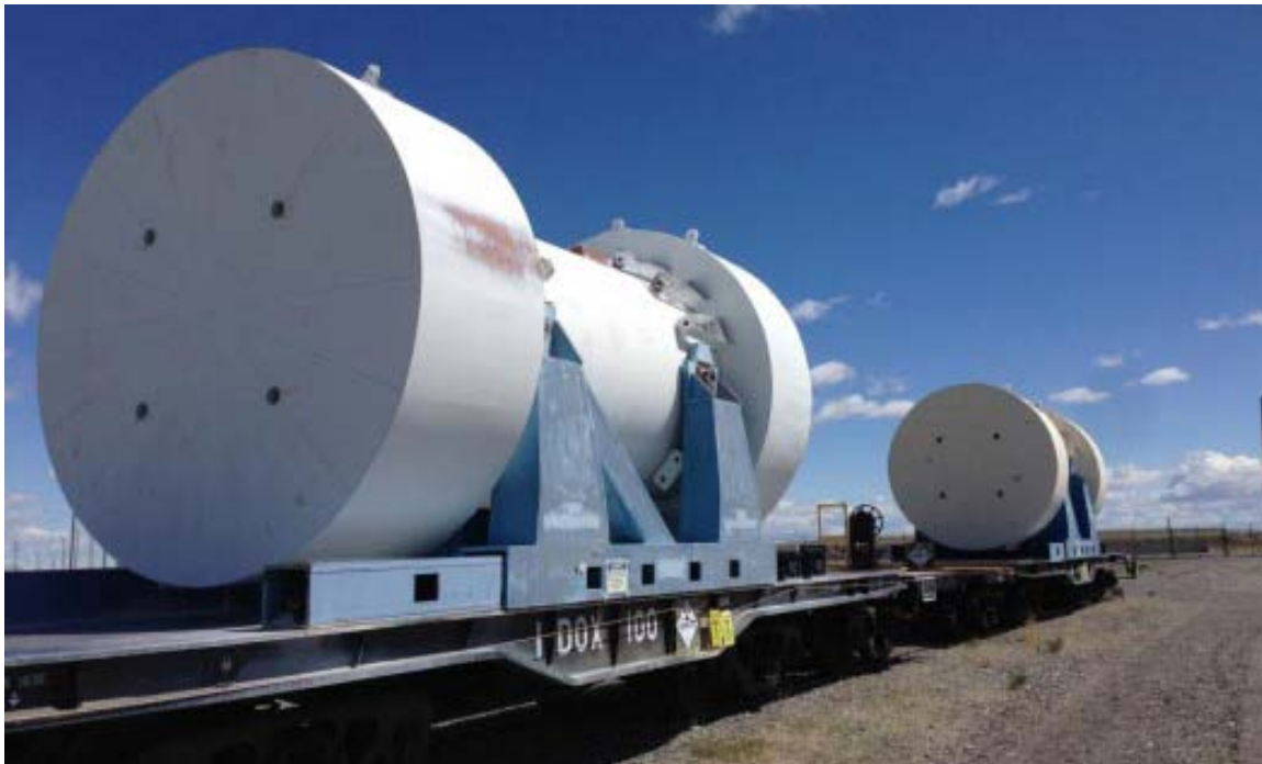
Figure ES-4. SNF rail transportation casks.
